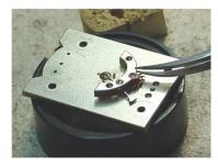
Fig. 39 Assembling escape wheel bridge
