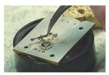
Fig. 38 Positioning escape wheel and fork
