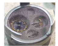
Fig. 27 Small parts on top, arranged to clear the lid
