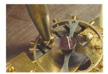
Fig. 42 Pressing in hairspring stud
