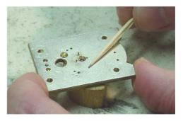
Fig. 28 Polishing the plates with the toothpick rub
