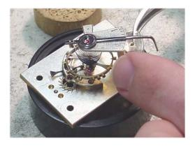
Fig. 45 Assembling balance cock to platform
