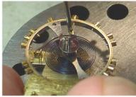
Fig. 43 Rotating regulator boot to capture hairspring
