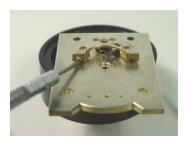
Fig. 20 Prying up escape wheel bridge
