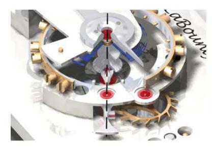
Fig. 49 Setting the beat using a sight reference (shown cut-away for clarity)
