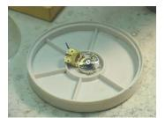
Fig. 16 Balance and cock in safe position
