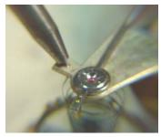
Fig. 18 Special punch to press out hairspring
