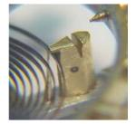
Fig. 44 Regulator boot in proper position
