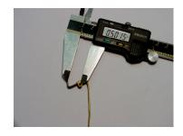
Divide that value in half and adjust a set of calipers to match. This value will produce a 2 degree lift angle. In half again will produce a 1 degree lift angle and so on. With this method, any angle may be produced.
