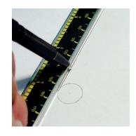
Use a smooth broach, or other sharp, tapered tool, and poke it through the paper in the exact center of the circle. Slide the pallets over the tool and rotate until the lift surface touches the line.
