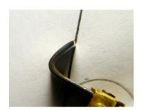
Use the jaws of a vise to help file off the proper amount and angle.
