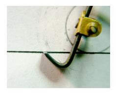
Finish the process by polishing the lift and lock surfaces to a mirror-like finish.
