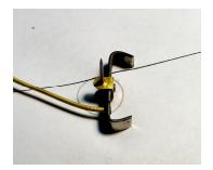
Examine both entrance and exit pallets to see if the angles are proper. Make a note of which portion of the pallet to file in order to correct the angle.
