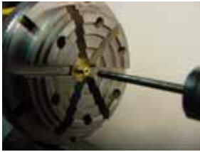
Shaving off the end for End-Shake
