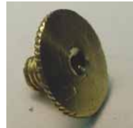
Repaired Hand Nut
