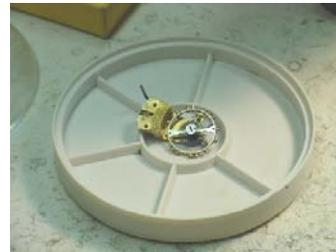
Fig. 16 Balance and cock in safe position
