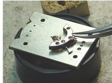
Fig. 39 Assembling escape wheel bridge
