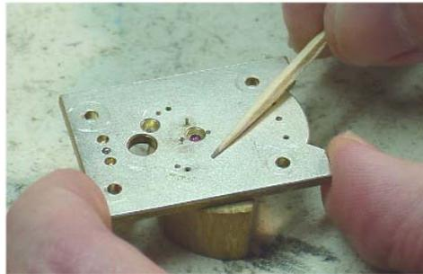
Fig. 28 Polishing the plates with the toothpick rub
