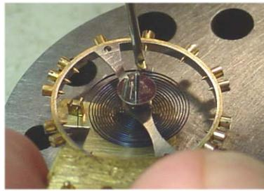
Fig. 43 Rotating regulator boot to capture hairspring
