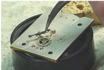
Fig. 38 Positioning escape wheel and fork
