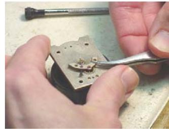
Fig. 21 Lifting escape wheel bridge straight up
