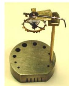
Fig. 48 Balance on balance tack for beat adjustment
