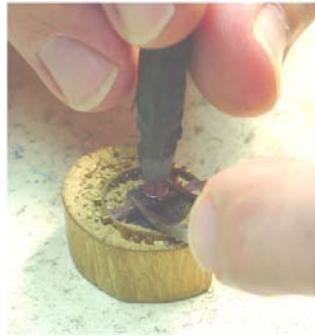
Fig. 23 Polishing pivots
