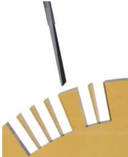
Figure 22: View of the count lever at its highest lift point during strike.
