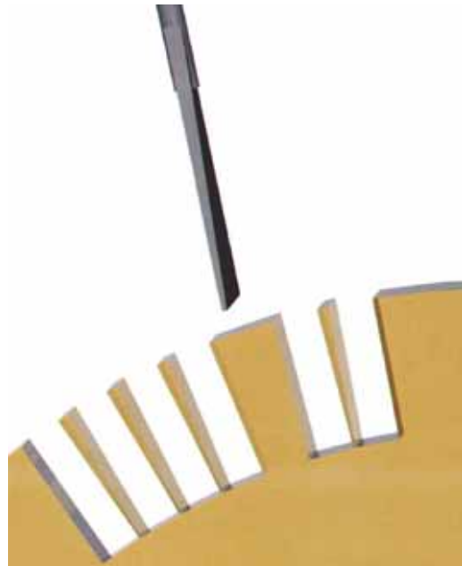
Figure 50: View of the count lever at its highest lift point during strike.
