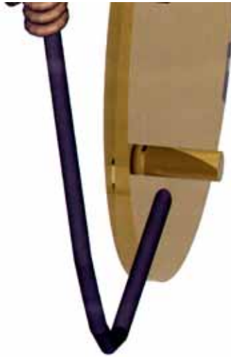
Figure 49: View of the closest approach of the warning pin to the warning lever during strike.
