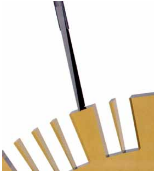
Figure 23: View of the count lever during strike resting on the rim of the count wheel and not in a stop notch.
