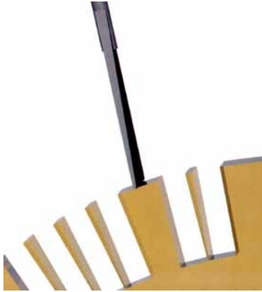
Figure 51: View of the count lever during strike resting on the rim of the count wheel and not in a stop notch.
