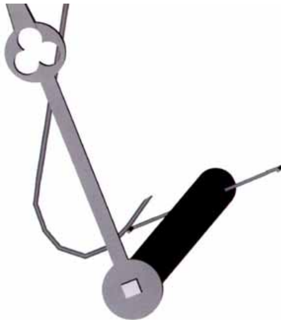
Figure 48: “J” lever and release pins in warning.
