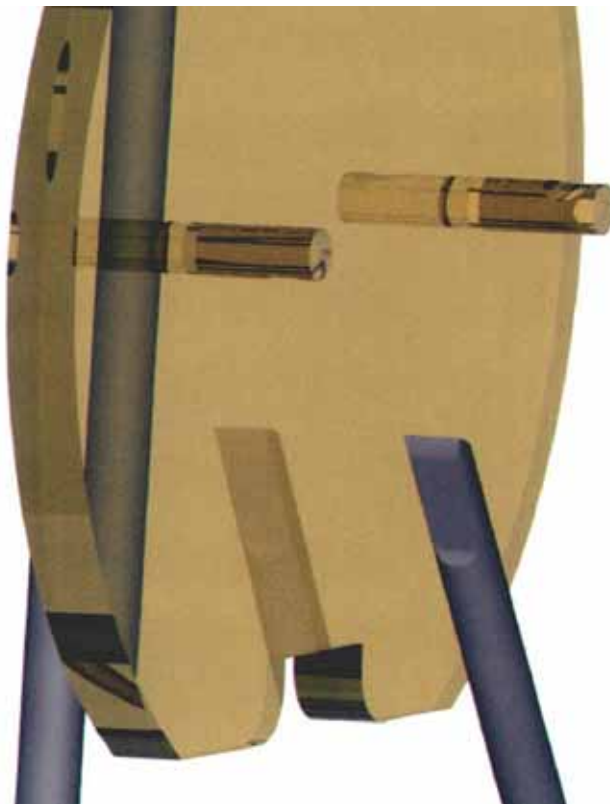
Figure 12: Wear on the hammer lever and hammer pins.
