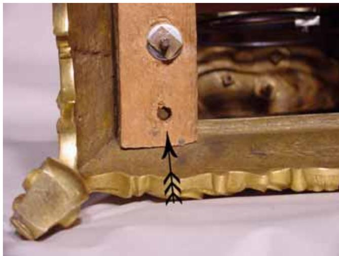
Fig. 3- Clocks with a repeat pull will generally have a hole in the case for the pull to pass through. This hole will also act as a guide and prevent the cord from becoming tangled in the movement (shown at arrow).
