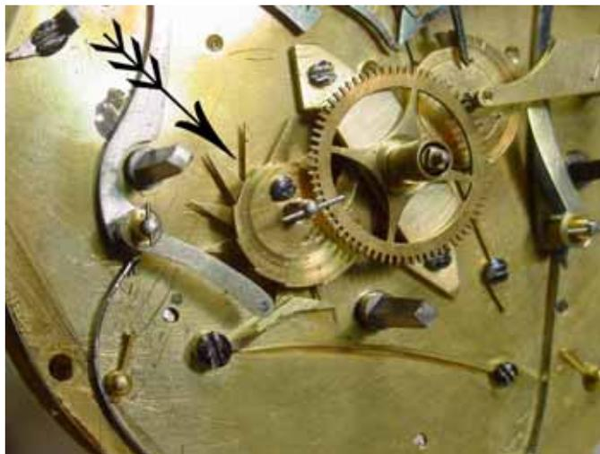
Fig. 1- A good indication of a repeat function is having the snail attached to a star wheel (shown at arrow).
