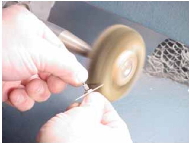
Fig. 21: De-burring the escape wheel teeth by spinning on the buffer. Note a brass brush is used to prevent damage to the wheel.
