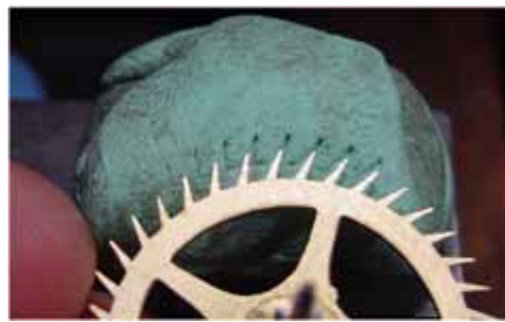
Fig. 12: Use the impression to compare the spacing of the teeth on the rest of the escape wheel.
