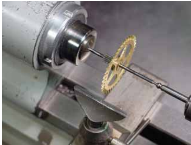
Fig. 13: Turning the escape wheel on the pivots will offer the highest degree of accuracy when tipping the escape wheel teeth.
