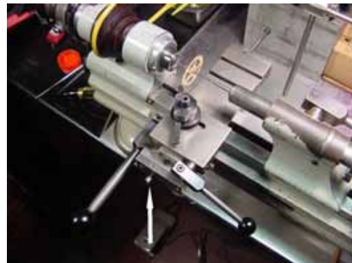
Fig. 17: Tipping with a lever feed cross-slide. Note the stop limiter at arrow which allows control of how much material is removed.
