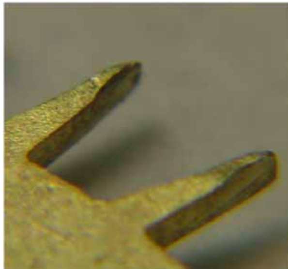
Fig. 4: Two escape wheel teeth showing slight damage. Note the irregular line along the tooth face, which can be easily seen with an eye loupe.
