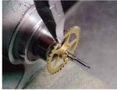
Fig. 7: Straightening a misaligned tooth.
