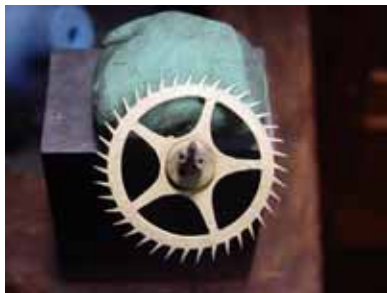
Fig. 11: Make an impression in the Rodoco of a section of good teeth to use as an indexing reference.
