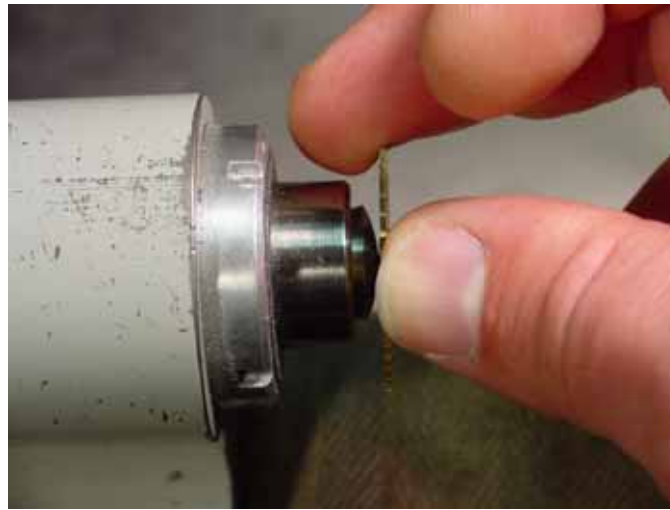
Fig. 8: Bringing the escape wheel back to true.
