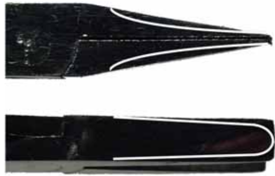
Fig. 3: A pair of flat-nosed pliers showing the areas to be relieved.
