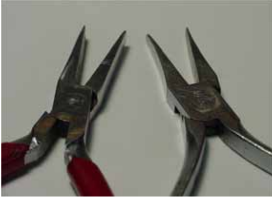
Fig. 2: A readily available pair of pliers (left) can be easily modified for escape wheel repair.
