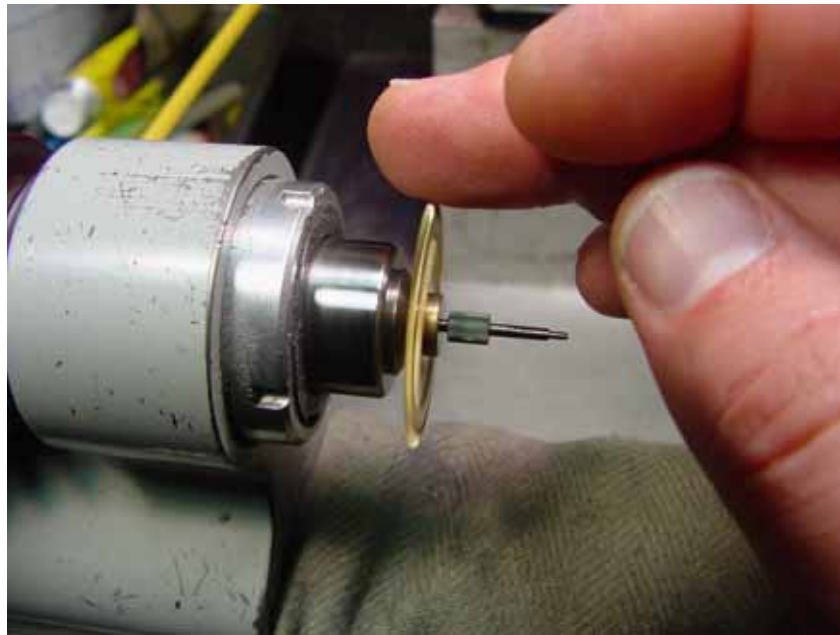
Fig. 5: A light touch on the edge of the spinning escape wheel, just prior to polishing the pivots, will allow you to feel a problem.
