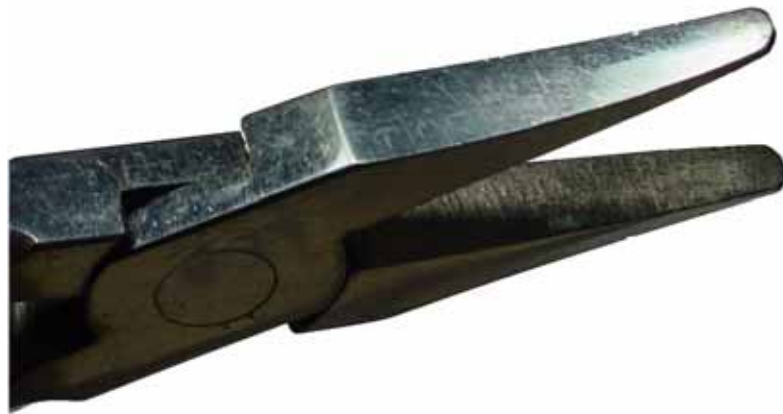
Fig. 1: A pair of pliers which will work well for straightening escape wheel teeth.
