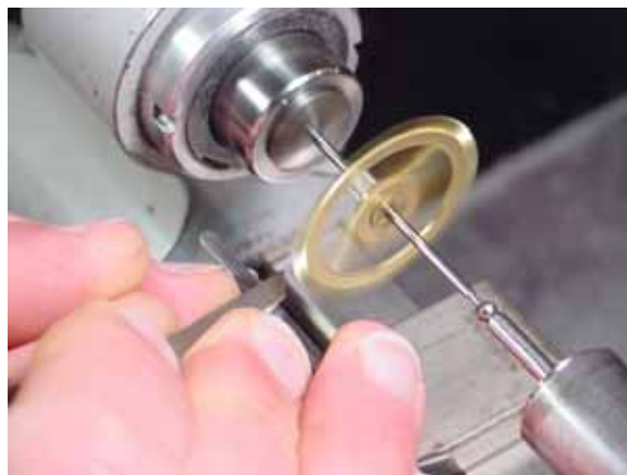
Fig. 15: Using a hand graver to tip the escape wheel to true.
