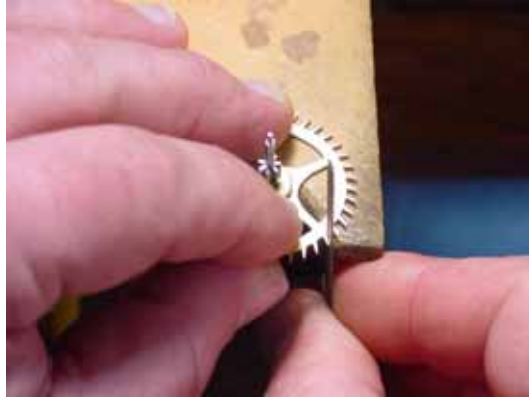
Fig. 22: Removing burrs by filing. Use consistent strokes to be sure each tooth is treated the same and support, support, support.
