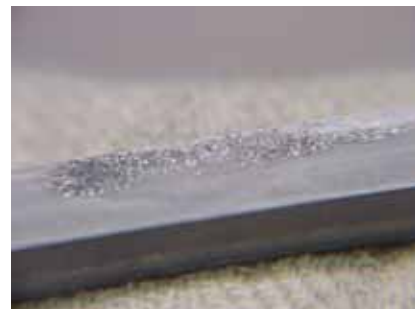
Fig. 1-Burnishing a plated pivot will cause the plating to flake, as shown here. The plating can be seen as particulates in the oil on the burnisher.
