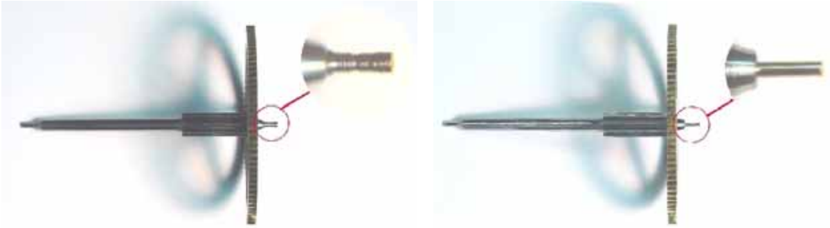
Fig. 36-An example of an “I” shaped pivot before polishing/burnishing (left) and after (right).
