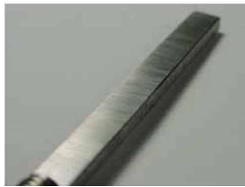
Fig. 18-Steel burnisher after prepping. There are no lines running the length of the burnisher and the finish is even.
