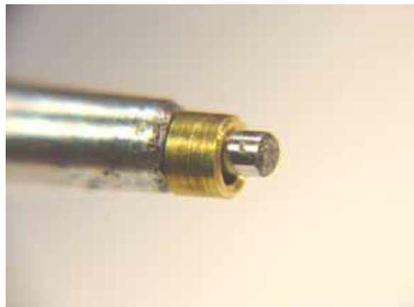
Fig. 35-If the defect in the pivot finish isn't on the bearing surface, there is no reason to reduce the diameter of the pivot in order to remove the defect. In this case, the defect is well beyond the pivot hole and can be left as is.
