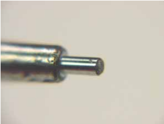
Fig. 34-Some imperfections on a pivot aren't necessary to be removed. The defect on the end of this pivot, for example, is a good candidate for one that can be left as is.
