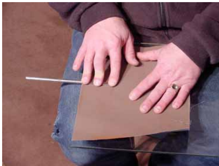
Fig. 21-Method of prepping a steel burnisher. Get comfortable, it may take a while.
