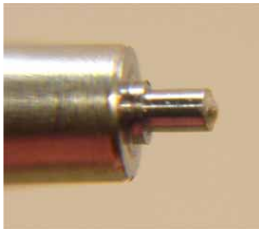
Fig. 40-Grinding a new shoulder, like this one, should be avoided when using the pivot polisher.
