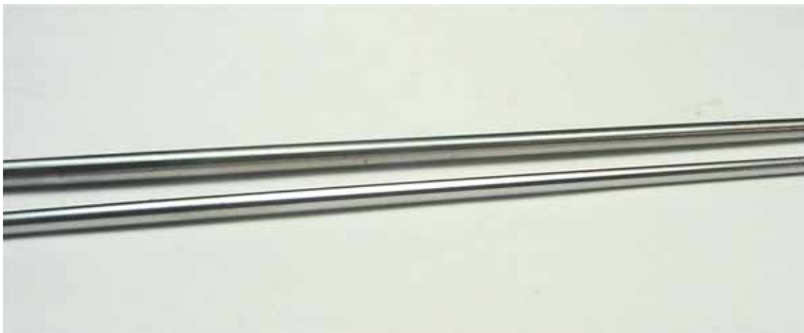
Fig 45-A new smooth broach, top, as compared to a freshly prepped one, bottom. Note: Even though the prepped smooth broach has a scratched finish, it has a brighter sheen than one which is not prepped. This shows the prepping process removes any contaminants that may be on a new, unprepped broach.
