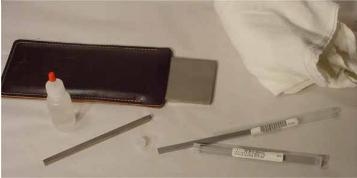
Fig. 22-Tools for making a carbide burnisher include kerosene, diamond lap 5 , diamond hone 4 , and a shop towel. The soon-to-be carbide burnishers are shown in the tubes 4 .
