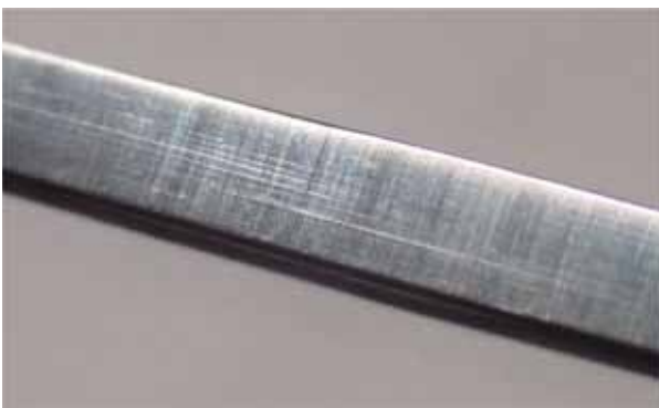
Fig. 17-A burnisher will need to be re-prepped if it develops wear lines. These will show up as lines running the length of the burnisher and can be clearly seen in the photo.
