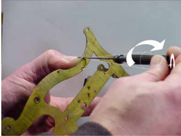
Fig 46-Wallowing a smooth broach to burnish a pivot hole is done by a combination of twisting the handle and articulating the broach in the pivot hole. This will afford a greater degree of “feel” while burnishing and minimize the amount to which the hole is made larger during the burnishing process.
