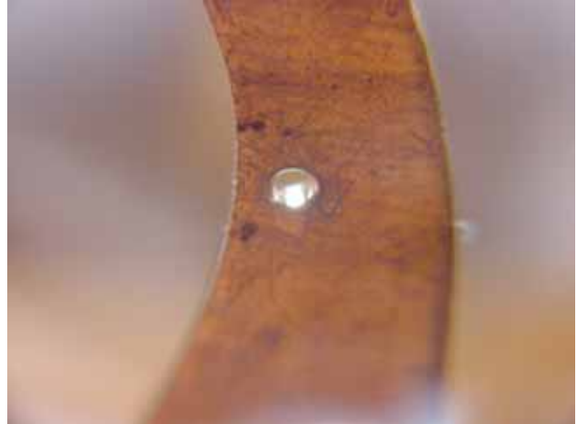
Fig. 48-After burnishing, the pivot hole is bright and shiny. A close examination of the plate, while being backlit, will quickly show if any pivot holes have been missed!
