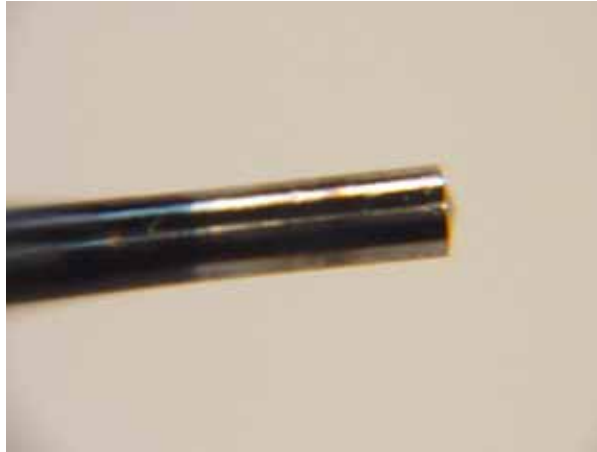
Fig. 39-Example of a burnt pivot (shown on pinion wire). Note the discolored, brown rings in the middle of the burnished area.
