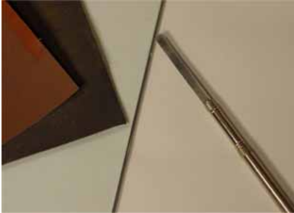
Fig. 19-Tools for prepping a steel burnisher include sandpaper and a thick glass plate.
