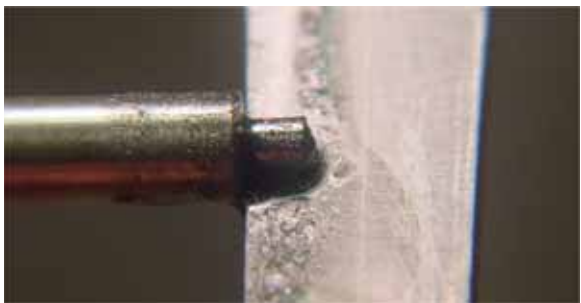
Fig. 1-Burnishing a plated pivot will cause the plating to flake, as shown here. The plating can be seen as particulates in the oil on the burnisher.
