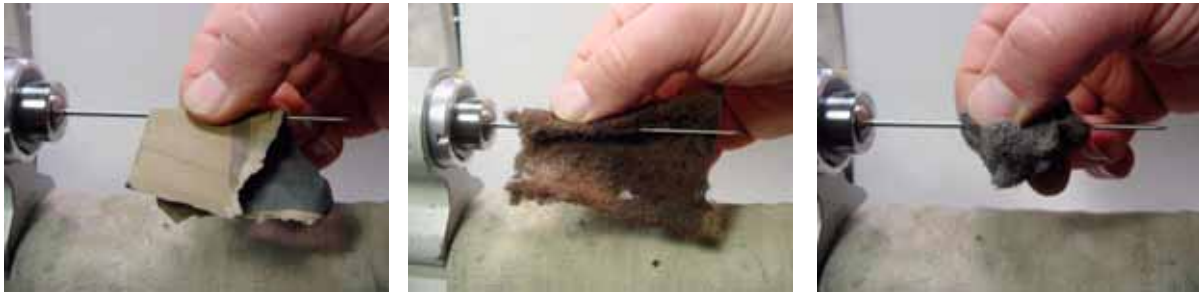
Fig. 42-Prepping a smooth broach may need to be done in several stages to obtain the optimal finish. Fine grit sandpaper, followed by Scotchbright and steel wool, produces a nice result.
