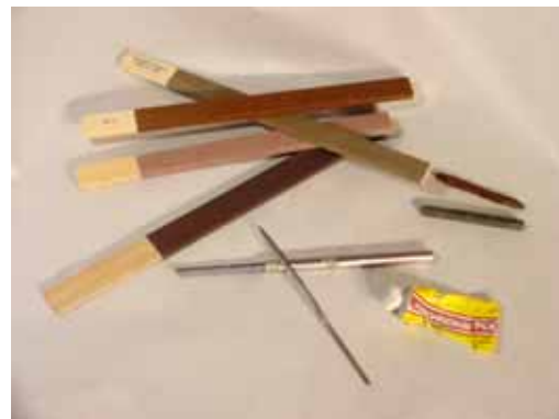
Fig. 4-An assortment of polishing aids includes buff sticks 1 , Craytex 2 , Simichrome 1 , and files.
