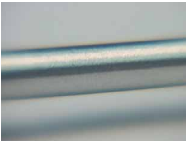
Fig. 43-The finish on a new smooth broach is unsuitable for burnishing and must first be prepped.
