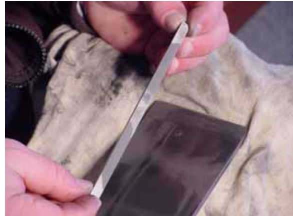
Fig. 26-After a short time of prepping, the burnisher will show where the high and low spots are. Once the whole surface of the burnisher is the same color, the prepping is done.
