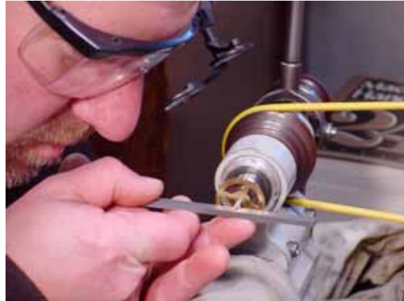
Fig. 31-Burnishing from underneath gives the craftsman visibility of the pivot. Since the work is very close, eye protection is a must.
