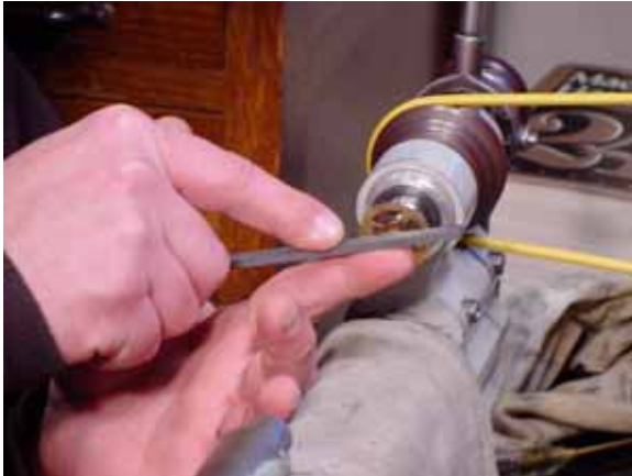
Fig. 30-Hand position for burnishing over-the-top. Note: The index finger is supporting the pivot and adding to the feel for keeping the burnisher flat.
