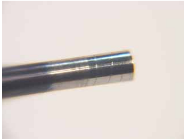
Fig. 33-A poor take-away of the burnisher will cause damage that is best to avoid. Shown here is the result of accidentally dragging the burnisher across the pivot as the burnisher is being taken away.
