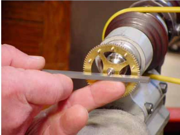
Fig. 32-Burnishing a pivot can sometimes be dangerous. It is best to know where the danger is and maintain a sure touch with the burnisher.
