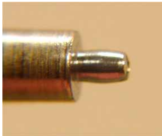
Fig. 6-Barrel shaped pivots are usually a result of poor technique. But this is sometimes done on purpose for specific movements.
