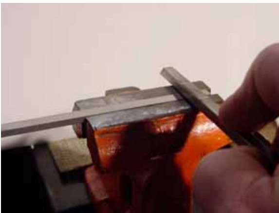
Fig. 27-Prepping the carbide burnisher with a coarse end using the diamond hone 4 .
