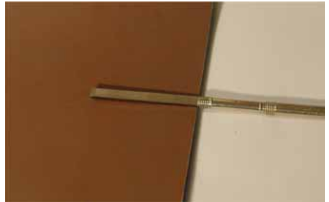
Fig. 20-Holding the edge of the burnisher handle against the edge of the glass will ensure the lines stay the proper direction.
