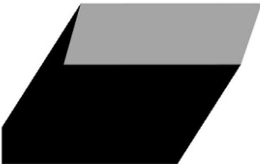
Fig. 8-Right-hand burnisher with an edge which has been relieved for top use with work on the right-hand side or beneath work on the left.
