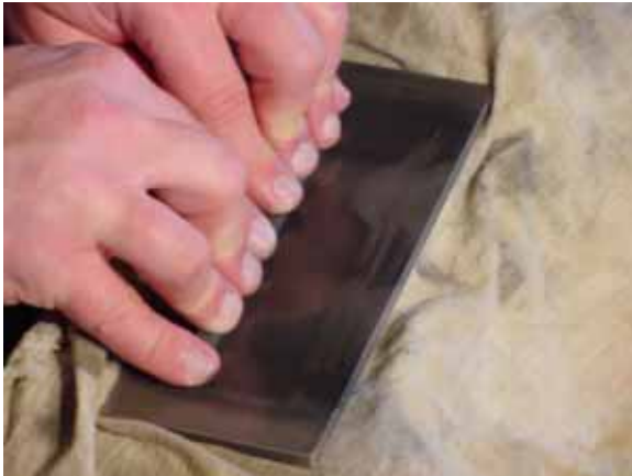
Fig. 25-Method of prepping. The back and forth motion must be carefully maintained so as to keep the lines on the burnisher running the proper direction.
