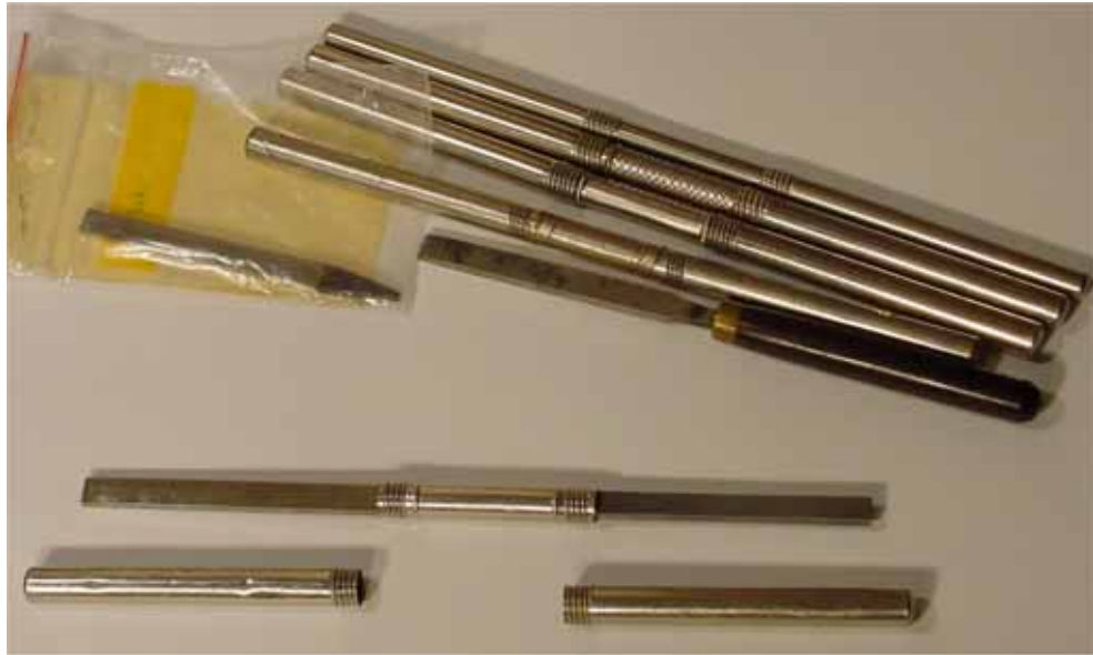
Fig. 16-Various steel burnishers and file/burnisher combos.
